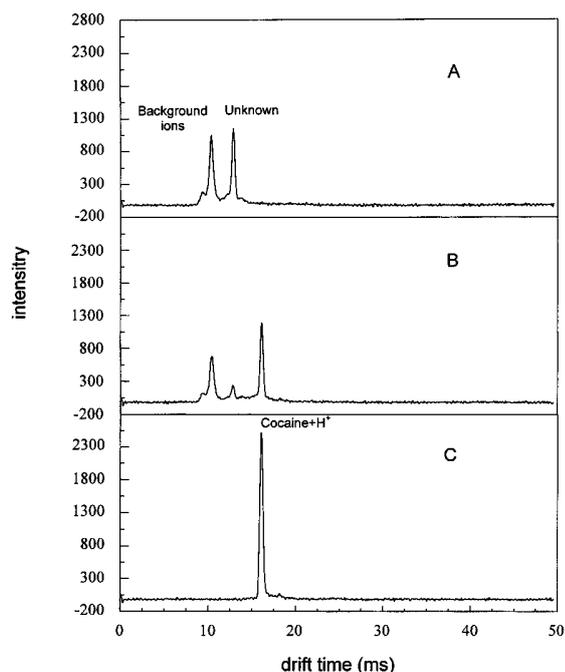
**Figure 8.** Ion-mobility spectra of cocaine by SESI-IMS after GC separation. Spectra A, B, and C are in order of GC elution time.
