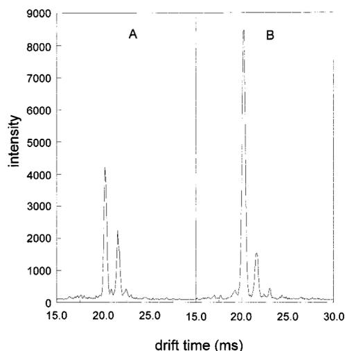
**Figure 9.** Ion-mobility spectra of cocaine with different sample flow rates with a secondary electrospray ionization source. (A) 5  $\mu\text{L}/\text{min}$ ; (B) 20  $\mu\text{L}/\text{min}$ . Higher ion intensity was detected at higher sample flow rate.
