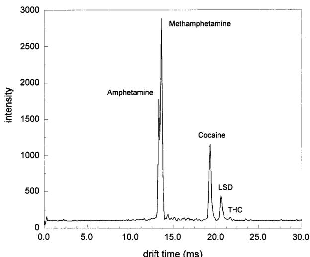
**Figure 3.** Ion mobility spectrum of a drug mixture ionized by an ESI source. A mixture of amphetamine, methamphetamine, cocaine, LSD, THC was prepared at a concentration of 11.5–23 ppm in methanol and water (1:1 v/v) with 1% acetic acid addition. Sample was introduced at a flow rate of 5  $\mu\text{L}/\text{min}$ . The ion-mobility spectrometer was operated at a total sampling time of 51 ms and a gate pulse width of 0.2 ms.
