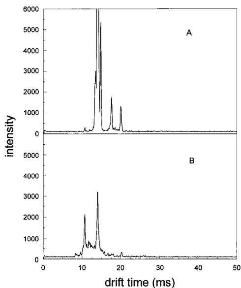
**Figure 7.** Product ions of amphetamine in the SESI source with different sample concentrations. (A) 1000  $\mu\text{g/mL}$ ; (B) 1  $\mu\text{g/mL}$ . Clusters form at a high sample concentration limited dynamic response range in the SESI source.
