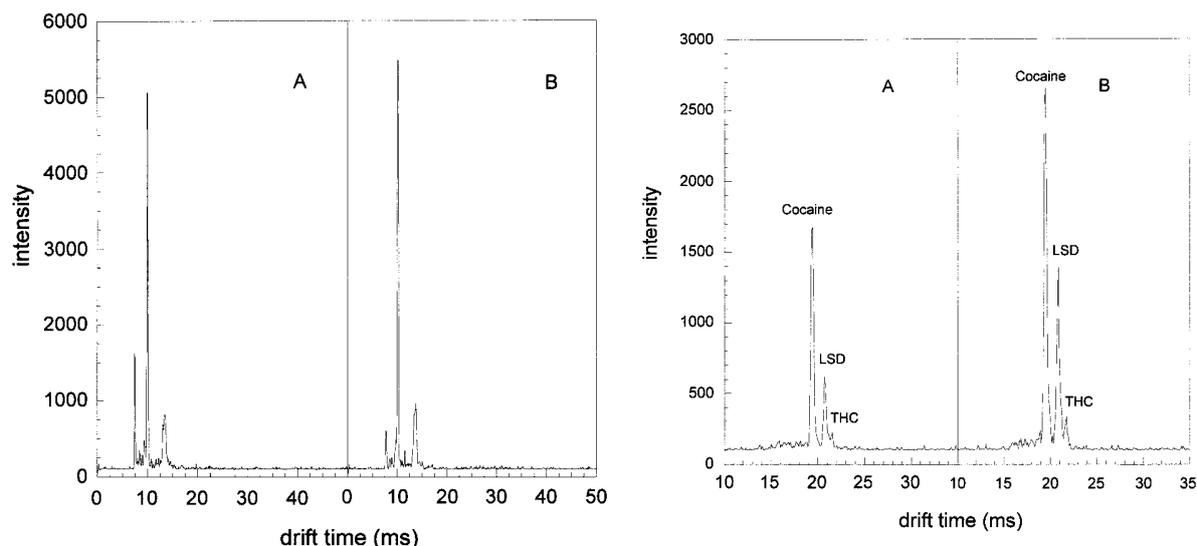
**Figure 4.** (a) Ion-mobility spectra of electrospray solvents (A) and that with addition of acetic acid from the gas phase (B). (b) Ion-mobility spectra of a drug mixture without vapor-phase acetic acid (A) and that with the addition of vapor-phase acetic acid (B). Mass-selective detection of  $m/z > 250$ . Detected ion intensity of the drug mixture was improved by 80% after addition of acetic acid in the gas phase.
