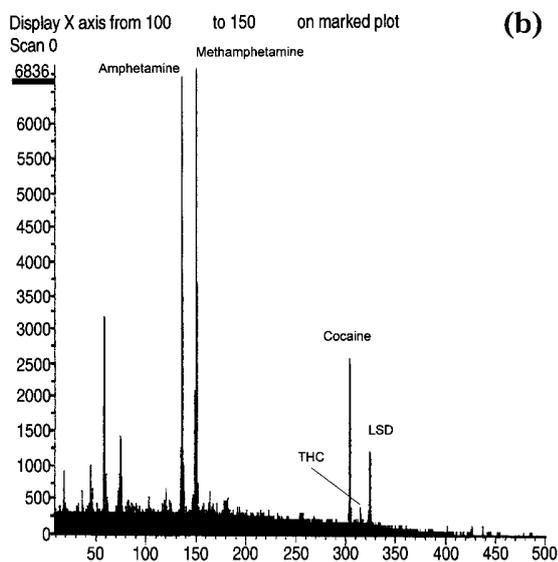
**Figure 5.** (a) Ion-mobility spectrum of a drug mixture ionized by an SESI source. Under the same operation conditions shown in Figure 3A, the drug mixture was introduced into the spectrometer from gas phase. (b) Mass spectrum of the drug mixture (same as shown in Figure 5a) ionized by SESI.
